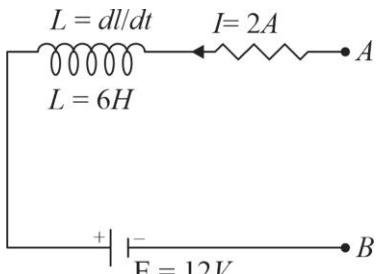
$$V_{AB} = V_R + V_L + V_E = +24 - 6 + 12 = 30V$$
