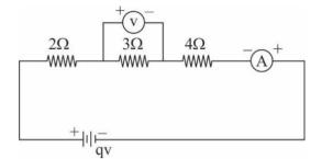
(i)  $R_S = 2\Omega + 3\Omega + 4\Omega = 9\Omega$ V = 9V
